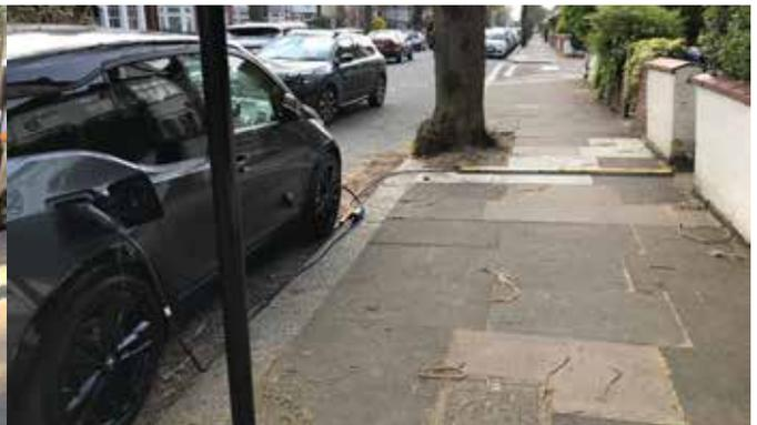
A pair of photos showing how the owner of this e-vehicle uses an adapted lamp column to charge the battery when they can get access to the kerbside in that location, and uses a trailing cable from their home when they cannot park near the lamp column.
