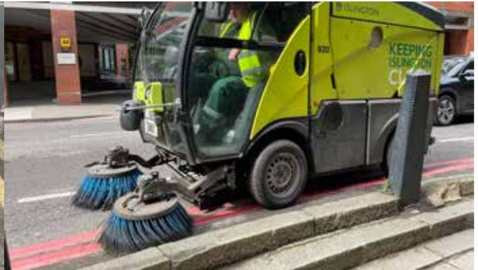
Easy access to the kerbside is needed for the purposes of sweeping and cleansing. This is often overlooked and/or difficult to enable.
