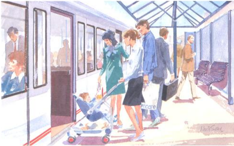
Profiled platforms will give level access to the front doors of trains.
