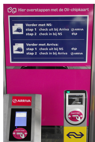
'Transfer point' on a railway platform, where passengers changing from Arriva to NS or vice versa have to touch out and to touch in again. These transfer points have been criticised for making the OV-chipkaart too complicated for passengers. Trials are currently (2015) being carried out with a 'single touch in – touch out' system for all railway operators, such as to be able to abolish these transfer points.
